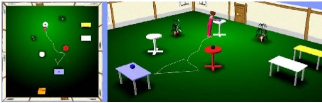
Fig. 11. “Migi no aoi tama wo kiroi tukue ni oke” (Pick up the blue ball of the right and put it on the yellow table.) Macro planner selected the blue ball from two blue balls and micro planner generated the path in detail. Natchan walks toward the blue ball and picks it up.
