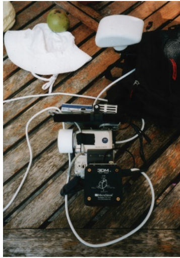
Fig. 4. Equipments; DV camera, PDA, GPS, and 3D strain
