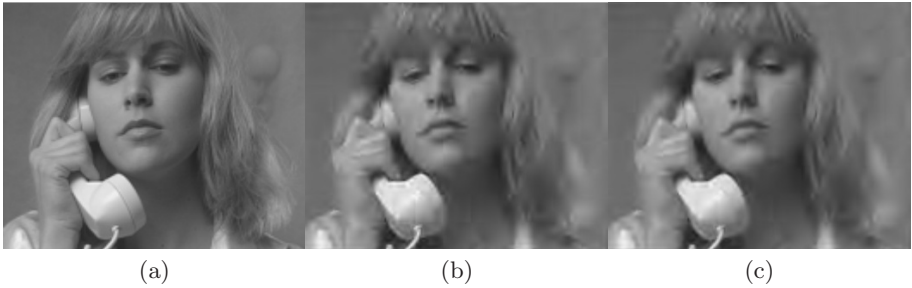
Fig. 3. (a) Original frame of the video (suzie), (b) the degraded frame by 3D wavelet video compression system and (c) the reconstructed frame by the proposed enhancement algorithm
