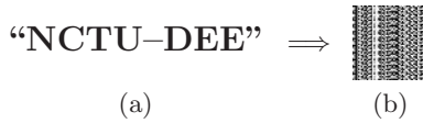
Fig. 3. Plaintext encryption and watermark generation. (a) The 8-byte plain-text. (b) The converted binary watermark with size 128 \times 128 .
