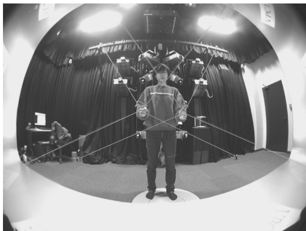
Fig. 4. A haptic interface “SPIDAR-H”. From motors to user’s hands, thin strings are strained to transfer torque generated with the motors.
